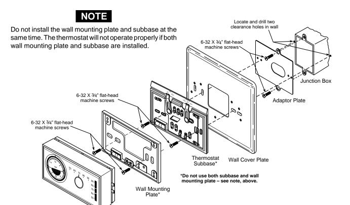
Figure 5. Mounting 1F7X quartz clock thermostat to vertical junction box
